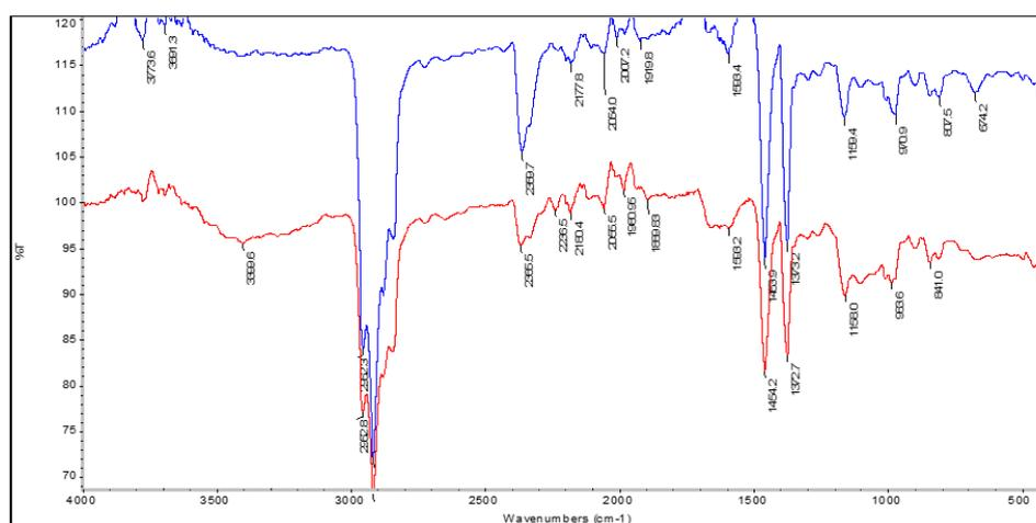
Fig. 1: FTIR result of Non-metalizedPP with control (Red) and treated with fungi ( Blue) spectrum.
