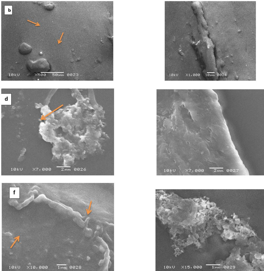
**Fig. 4:** SEM photomicrographs of Non-metalized cpp film exposed by *Aspergillus spp* and *Pencillium spp* (a)500x (b)1000X (c)7000x (d)10,000x (e)15000x respectively after 30 days of incubation
