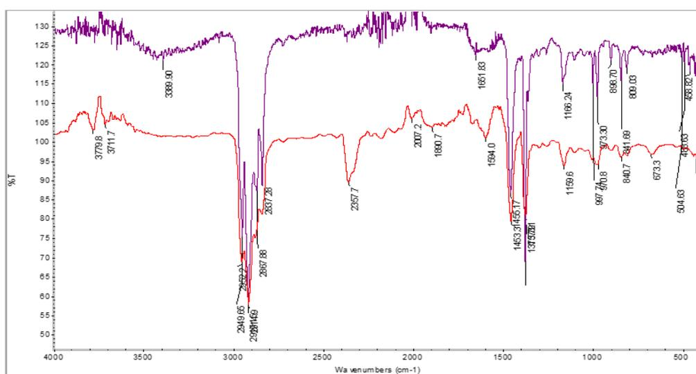
**Fig. 2: FTIR analysis result of metalized (red spectrum control) and metalized film (purple spectrum) after treated with fungi.**
