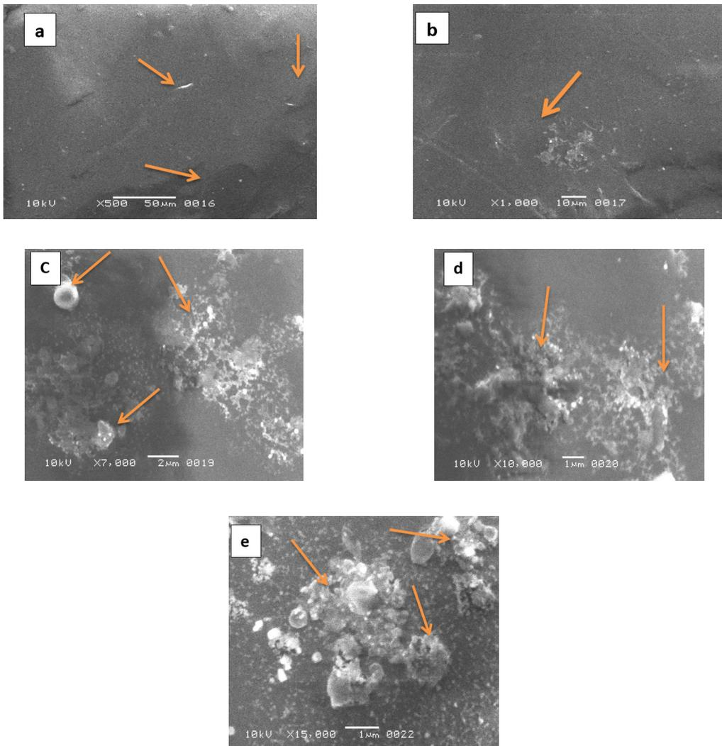
**Fig 3: SEM photomicrographs of metalized CPP film exposed by *Aspergillus spp* and *Pencillium spp* at (a) 500x (b) 1000x (c) 7000x (d) 10,000x (e) 15,000x respectively after 30 days of incubation**
