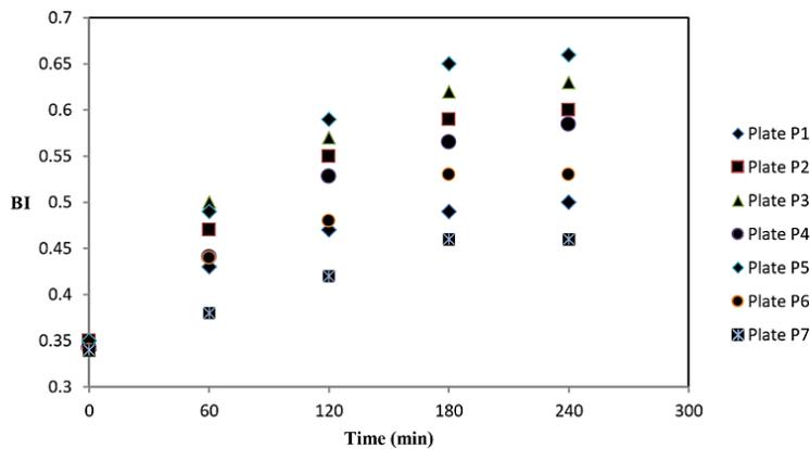
**Fig. 3: Influence of orifice plate geometry on the improvement of wastewater biodegradability at an inlet pressure of 2 bar.**
