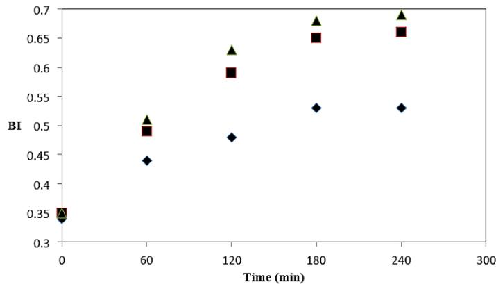
**Fig. 5: Effect of pH on biodegradability index of waste water at inlet pressure of 2 bars, orifice plate P5 and temperature of 30°C**
