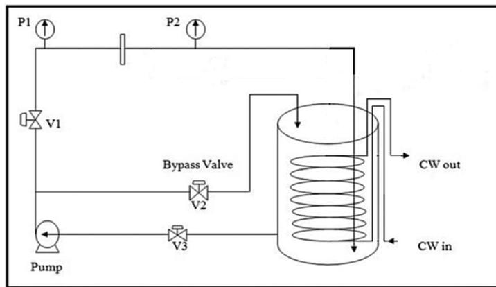
**Fig. 1: Schematic flowchart of hydrodynamic cavitation setup**
