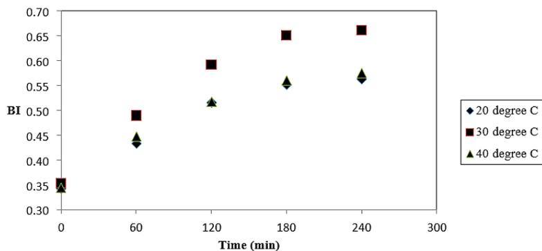
**Fig. 4: Effect of temperature on Biodegradability index at inlet pressure of 2 bars with orifice plate P5.**
