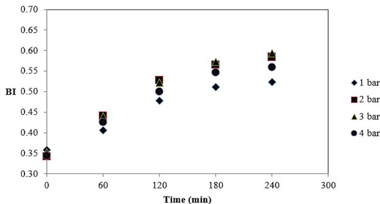
Fig. 2: Effect of inlet pressure across the orifice plate on the enhancement of the biodegradability index (BI) of dairy wastewater
