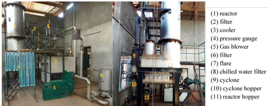
Fig. 1: Biomass gasification plant of Songhai Center located in Porto-Novo, Benin
