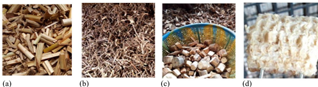
Fig. 4: Feedstock used in this work, (a) Corn stalks, (b) Cotton stalks, (c) Acacia auriculiformis Wood, (d) Corn cobs
