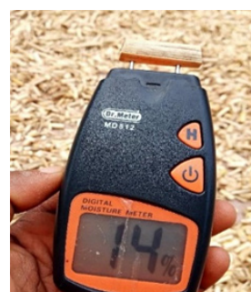
Fig. 6: Checking the moisture content
