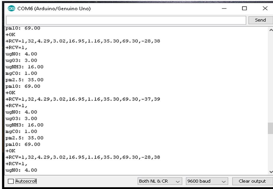
Fig. 6: Com-port Image of LoRa Receiver Module at Base Station
