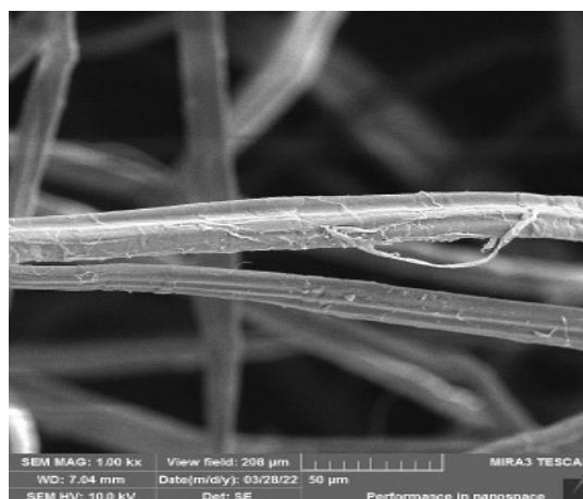
Fig. 7(b): SEM view of treated PJ fibers
