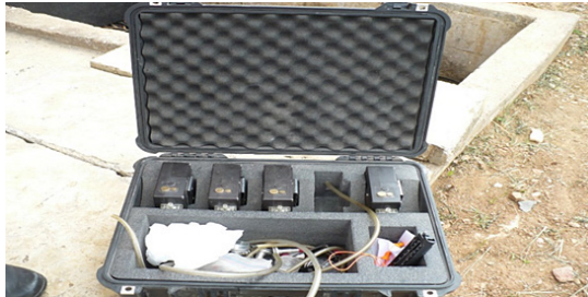
Fig. 3: Dust sampling kit
